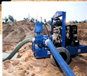
Diesel engine driven self-priming pump mounted on site trailer
