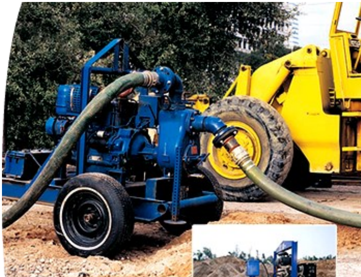
Diesel engine driven self-priming pump mounted on site trailer
