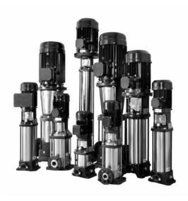
The VMS Series is a vertical in-line multistage centrifugal pump which is driven by a standard electric motor. The motor output shaft directly connects with the pump shaft through a coupling. The inlet and outlet are located at the pump bottom at the same plane.
